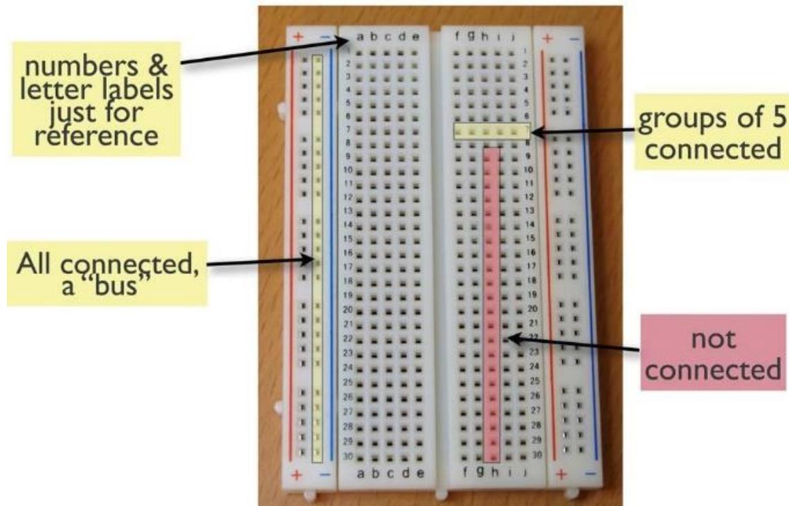
2) Some breadboards have a break or small separation in the middle of the power rail rows. If your board is like that, put a wire in a hole on one side of the break and the other end of the wire on the other side of the break. That will connect both sides. You'll need to do that for all four rails.
