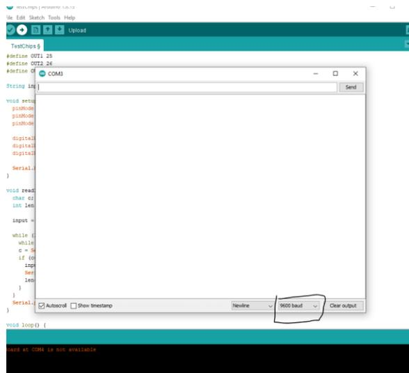
5. Once this window has been opened, press the reset button switch labeled EN. This will cause the board to reset. Follow along with the instructions to change ESP32 outputs to input into your circuit
