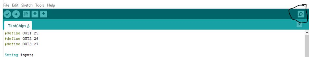
4. This will open the serial monitor, make sure that the baud rate (lower right) is set to 9600 baud
